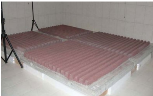
Figure 2. a) Real scale test samples in the reverberation room [7]
