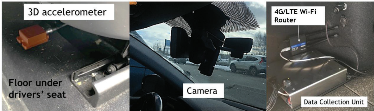
Fig. 1. Components of the basic RDMC system. 3D accelerometer is installed under the driver's seat and camera in front window. Data collection unit working with 12V DC can be in the trunk as well as GPS and 4G/LTE antenna. The system can be set to measure when the vehicle is running, or it can be started by cell phone.
