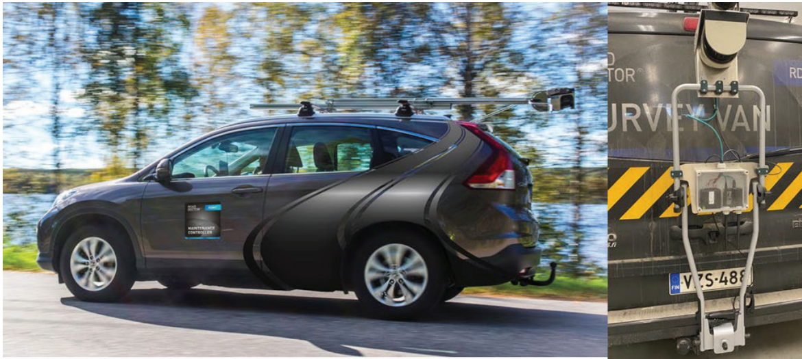
Fig. 6. RDMC laser scanner system can be quickly installed either to the roof or to the tow hook using a suitable rack.
