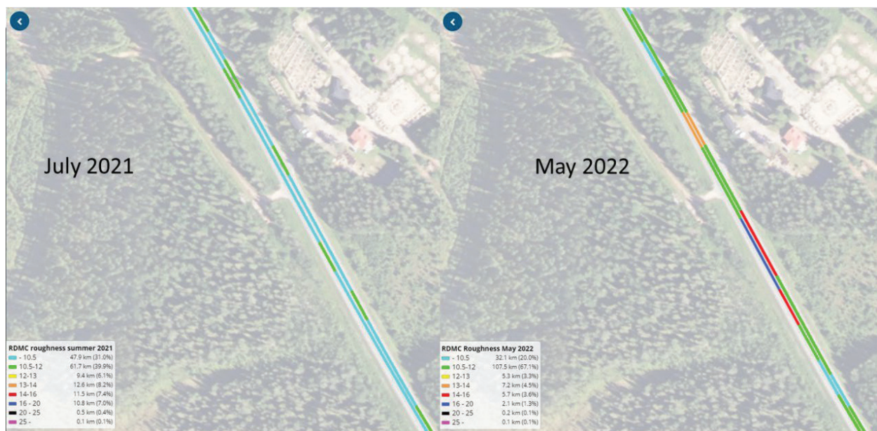
Fig. 10. Maximum vertical acceleration on Road 79 in Finnish Lapland measured in July 2021 when there was no frost and in early May 2022 during the frost thawing phase.
