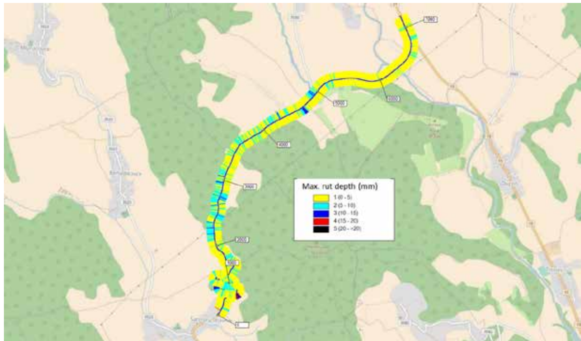
Figure 9. Laser scanner data interpretation showing maximum rutting results on a GIS map ( www.openstreetmap.org ).
