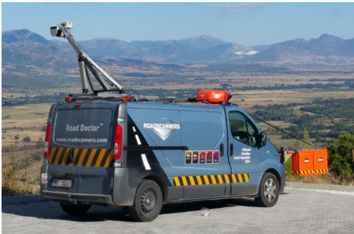
Figure 1. Road Doctor Survey Van. Two 2 GHz GPR antennas in the front, in coreless setup. Video camera on the roof and laser scanner at the rear (at 3 m) with GPS/IMU-positioning unit. Accelerometer is attached to the rear axle.
